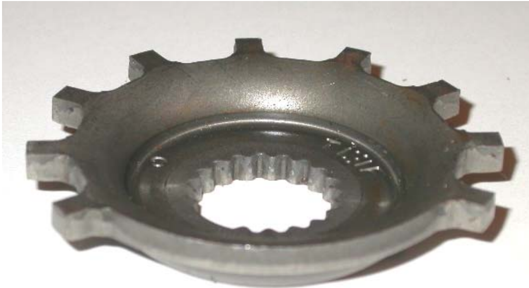
Figure 2 – Stock Honda F2 Trigger Wheel
