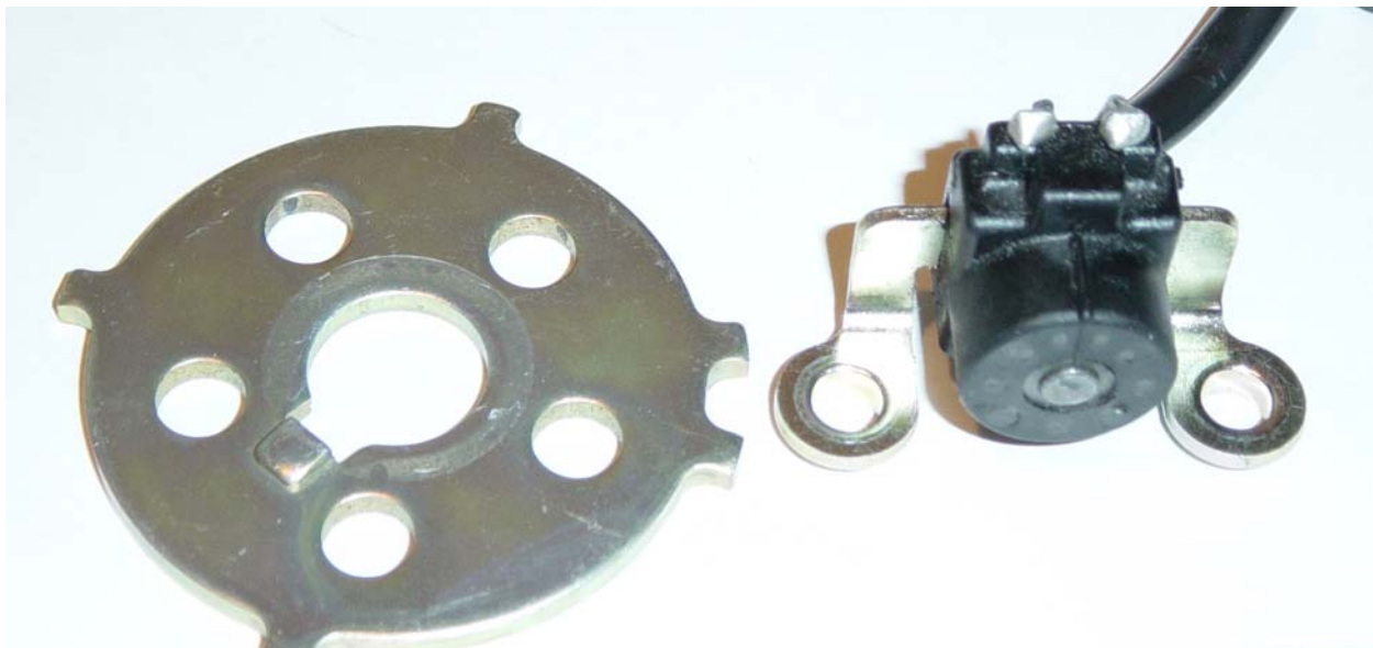
Figure 1 – Approved Yamaha Sensor and '99 – '02 R6 Trigger Wheel
